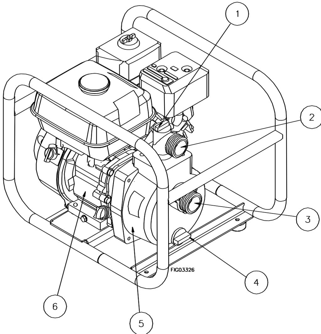
1. **Prime Port:** Fill the priming port to prime the pump.
