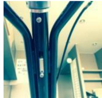
5. Install the wire to the Yoke Arm (Handle parts diagram, item 24) and tighten the nut.
