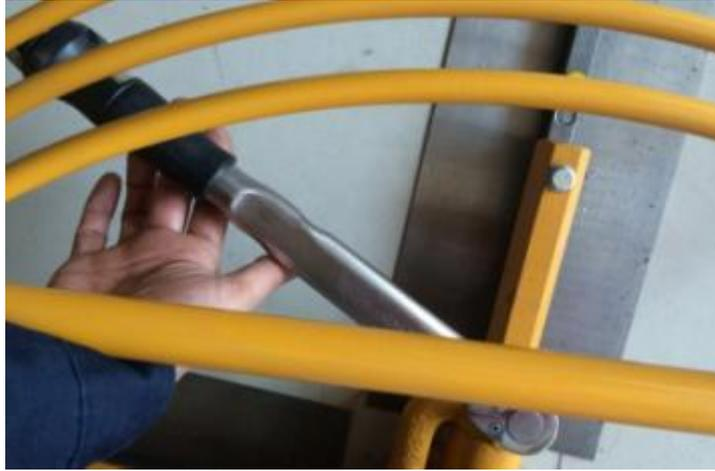
9.2 Keep the torque wrench setting at 13.02 ft-lb and tighten the outer bolt (Fig. 5).
