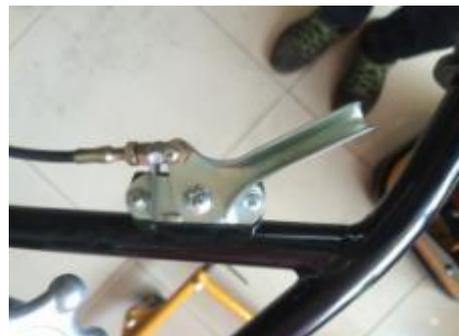
8. Check that the engine throttle lever (silver lever in picture) is at its idle position (fully left in picture) then attach the Accelerator Cable position (3) and wire (4).
