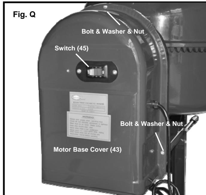
22. The Cement Mixer assembly is complete. Go back and retighten all screws, nuts, and bolts.
